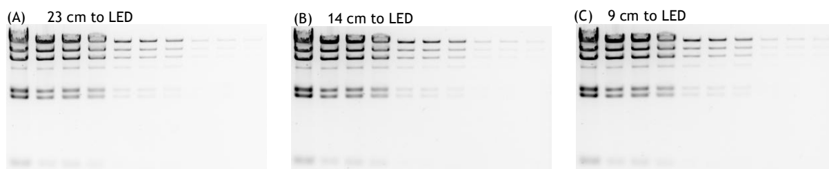
Figure 3. Epi-Blue LED excited SYBR Gold stained agarose gel in KETA ML with 0.2 seconds exposure time. Place the gel with (A) 23 cm, (B) 14 cm, and (C) 9 cm in distance to LED lights.
